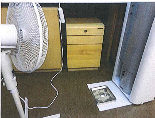
Picture 1. Lyophilized preparation of four target organisms on a tray was used to contaminate the air.
