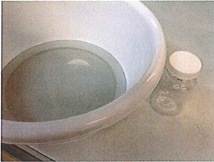
Picture 3. The washing liquid of the purifier after the use for purifying the air artificially contaminated with different microbes. The liquid was cultured for the determination of target organisms.
